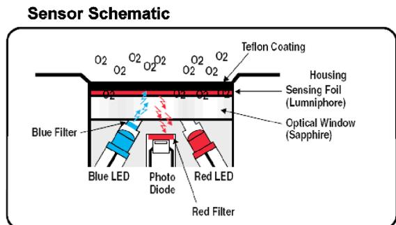
Optical DO Measurements are based on selected substances that can act as dynamic fluorescence quenchers. For example for oxygen, if a ruthenium-complex is illuminated with a blue LED it is excited and emits back a red luminescent light with an intensity, or lifetime, which directly depends on the oxygen concentration. Lifetime based measurements are superior for both long-term (no drift) and fast response applications.
